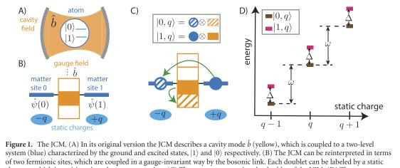
charge *q*, which is positioned on the two matter sites. (C) The two states spanning the doublet of the JCM. (D) The gauge invariant coupling leads to the formation of doublets in the Jaynes–Cummings ladder.
